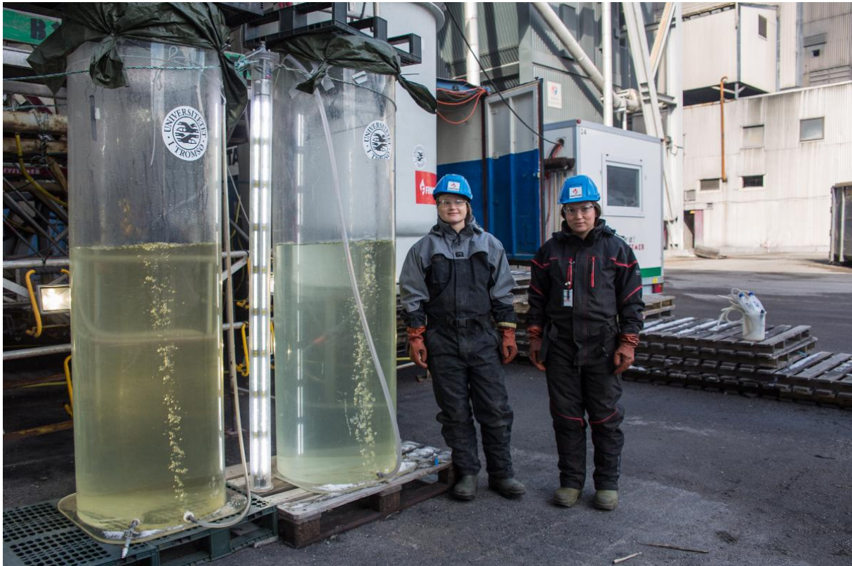
Figure: Small-scale incubators/tanks for algae production at Finnfjord. Photo: Tommy Hansen, UiT.
