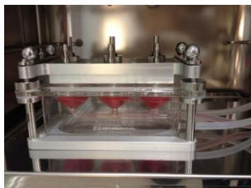
Figure 2. CULTEX device for ALI exposure of lung cells. The nozzle shape ensure even distribution of the aerosol to the cell layer. Circulating water keeps temperature constant.
