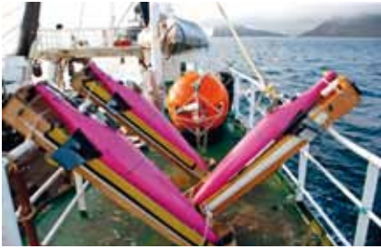
These robotic, free-maneuvring Seagliders, developed by the University of Washington, help researchers to collect a variety of oceanographic data. (Photo: private)
