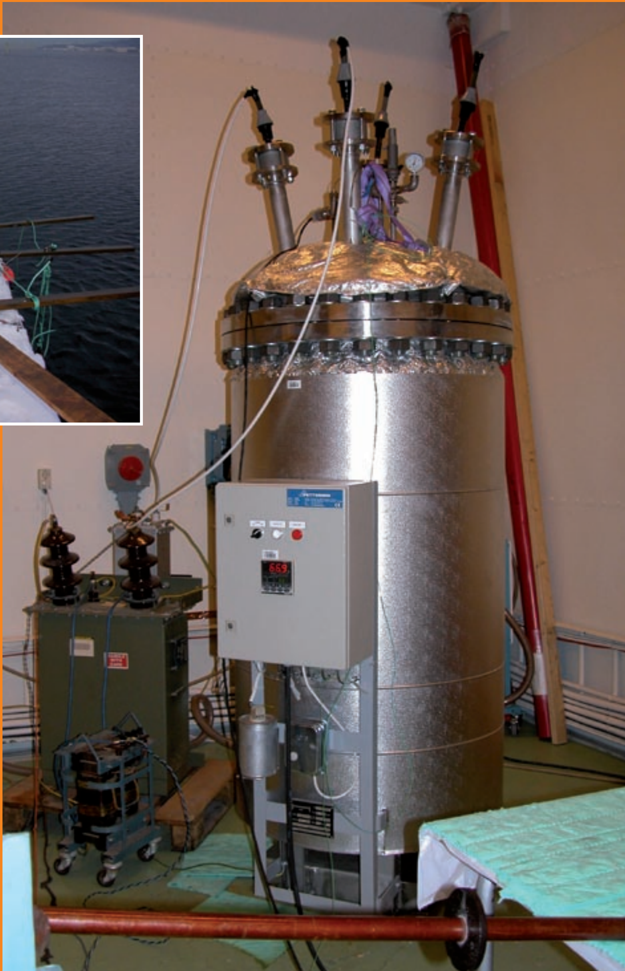
Lifetime testing of cables under pressure and voltage. In the laboratory tests are carried to see how long the cables can withstand damp conditions under a certain pressure and voltage. Photo: Hallvard Farmo.
