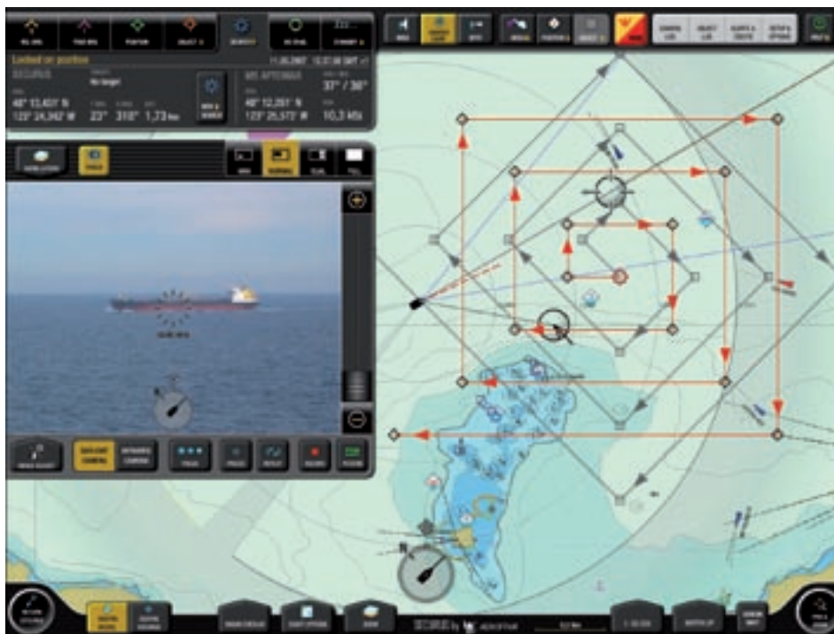
Aptomar uses advanced data systems technology, radar and IR cameras to give accurate positional information to ships and other installations, in addition to the thickness and spread of possible oil spills. Coordination of all the information in real-time will make clean-up and damage limitation safer and more efficient.
